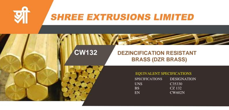
Alloy CW132 Brass is a copper-zinc-lead alloy with a small addition of arsenic, having a mainly alpha phase structure in the "as used" heat treated condition, with a fine dispersion of lead particles. It has excellent machinability, good cold forming properties, with a high resistance to dezincification.
