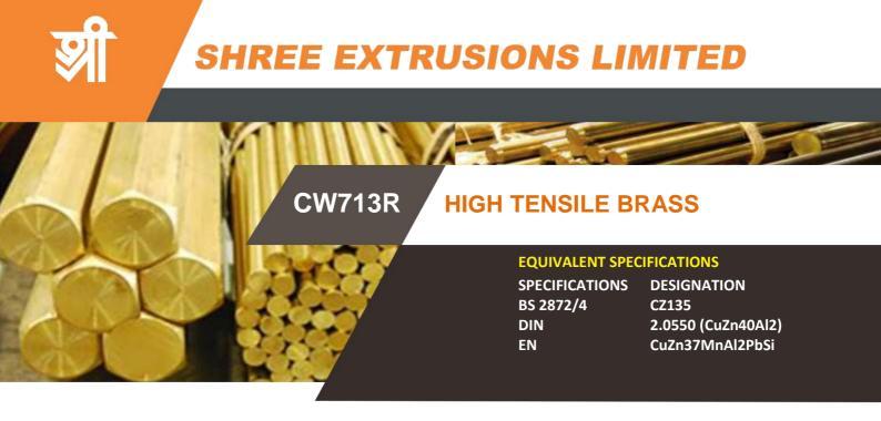
CW713R is a high tensile brass which is alloyed with aluminum, manganese and silicon etc. which makes this alloy almost as hard as aluminum bronze, but considerably easier to process. CW713R also has good corrosion, wear resistance and machinability.
