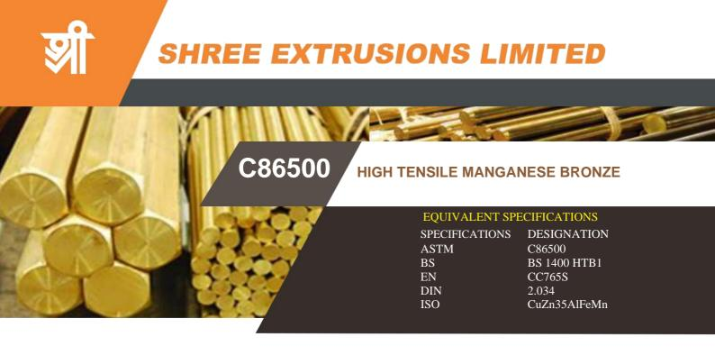
**C86500 High Tensile Manganese bronzes** high strength copper-based alloys that include manganese as an alloying agent and high levels of zinc. They are characterized by high strength and hardness. This grade provides tensile strength to 110,000 psi and hardness well over 200 BHN. Manganese bronzes are used for trunnion bearings, heavily stressed gears, gearshift forks, impellers, marine propellers, valve stems, worm gears, and worms. It is also used for highly stressed machine parts.
