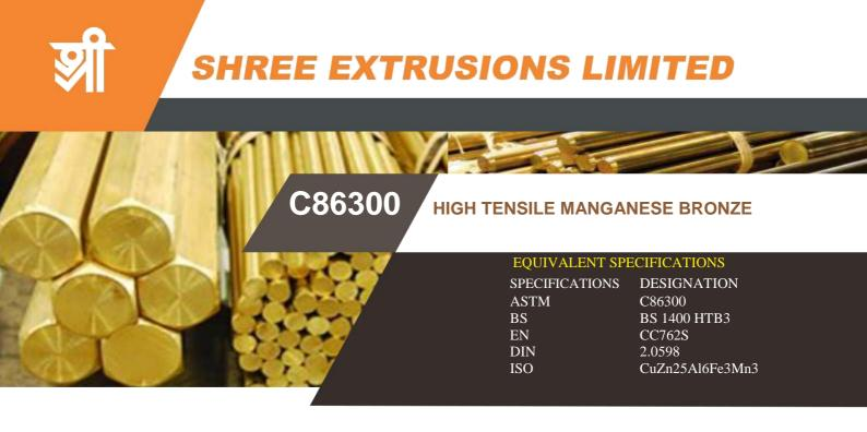
**C86300 High Tensile Manganese Bronze** is ideal for high load, low speed applications that require a combination of outstanding wear characteristics and high bearing strength. Despite its strength characteristics, however, this manganese bronze alloy is not heat-treatable, needs reliable lubrication and should be used in conjunction with hardened shafts. The lead in the alloy's makeup improves machinability without materially affecting its mechanical properties.
