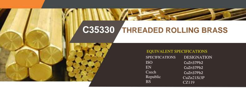
Excellent hot and cold workability; good forge ability. Fabricated by bending, coining, coppersmith, drawing and upsetting, hot forging and pressing, knurling, roll threading, shearing, spinning, swaging, and stamping.
