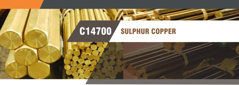
C111 / CW114C is a free machining sulphur copper with a machinability rating of approximately 80% (free machining brass = 100%). The addition of sulphur to the copper creates Cu2S copper sulphide within the microstructure that acts as a chip breaker and forms the basis of the free machining capacity.
