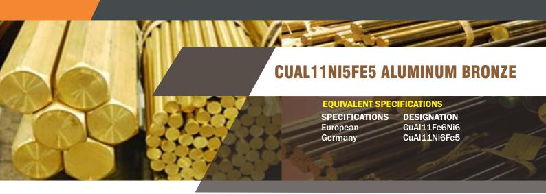
CuAl11Ni5Fe5 is an excellent choice for its application on aeronautical industry, due to its high mechanical properties and oxidation resistance. CuAl11Ni5Fe5 is resistant to corrosion in saline mist area
