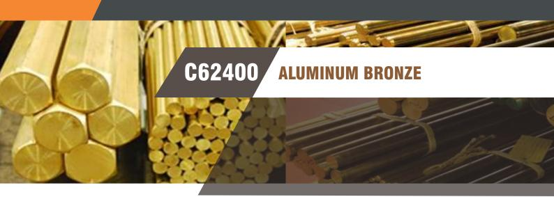
C62400 aluminum bronze applications include valve and pump components for industrial process streams, as well as for marine equipment, high strength fasteners and pole line hardware.
