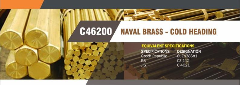
C462 brasses are very useful because of their strength, ductility & formability, fair electrical conductivity, and good corrosion resistance. Common applications for brasses include forged, stamped, rolled, and cold-headed products for electrical, mechanical or corrosion resistant applications. Due to their colorful nature, brasses are often used for decorative and architectural products and marine hardware.
