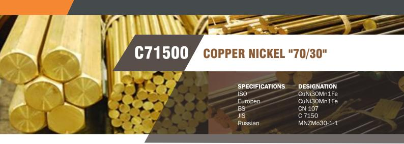
C71500, Copper nickel offers excellent corrosion resistance, especially in marine salt water environments. The main, wrought coppernickel alloys chosen for sea water service contain 10 or 30 percent nickel. They also have important additions of iron and manganese which are necessary to maintain good corrosion resistance. Some common applications for copper nickel include: valves, and pump components.
