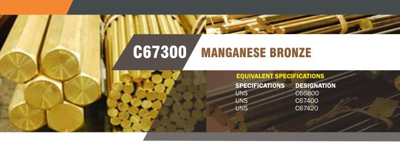
This is a high strength leaded silicon manganese bronze with typically good bearing qualities. This alloy maintains high impact resistance with excellent machinability making it well suited for clutch bearings, shaft bushings, sleeve bearings, thrust bearings, pump parts, drive shafts, bearing pins, wear plates, gears and cams. Resists squashing out under high loads and extreme wear applications.
